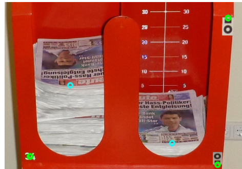
Fig. 1. Detection of markers and the box id (green circles) and the estimation of the paper stack limits (blue circles).
