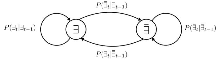
**Fig. 3.** Transition model to predict the current probability of existence before it is updated with new measurements
