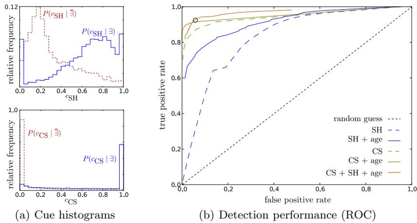
**Fig. 4.** Distribution of the three cue values for real obstacles and phantoms (a) and the resulting detection performance shown as ROC curve (b). The term "age" denotes temporal filtering here
